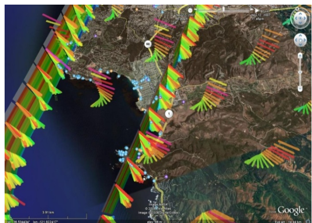
Figure 9 – Juxtaposition DWL wind cross sections with 4km MM5 meso-scale model output for same time period. The MM5 does not resolve low-level wind shear associated with fine scale flow about the local terrain.
