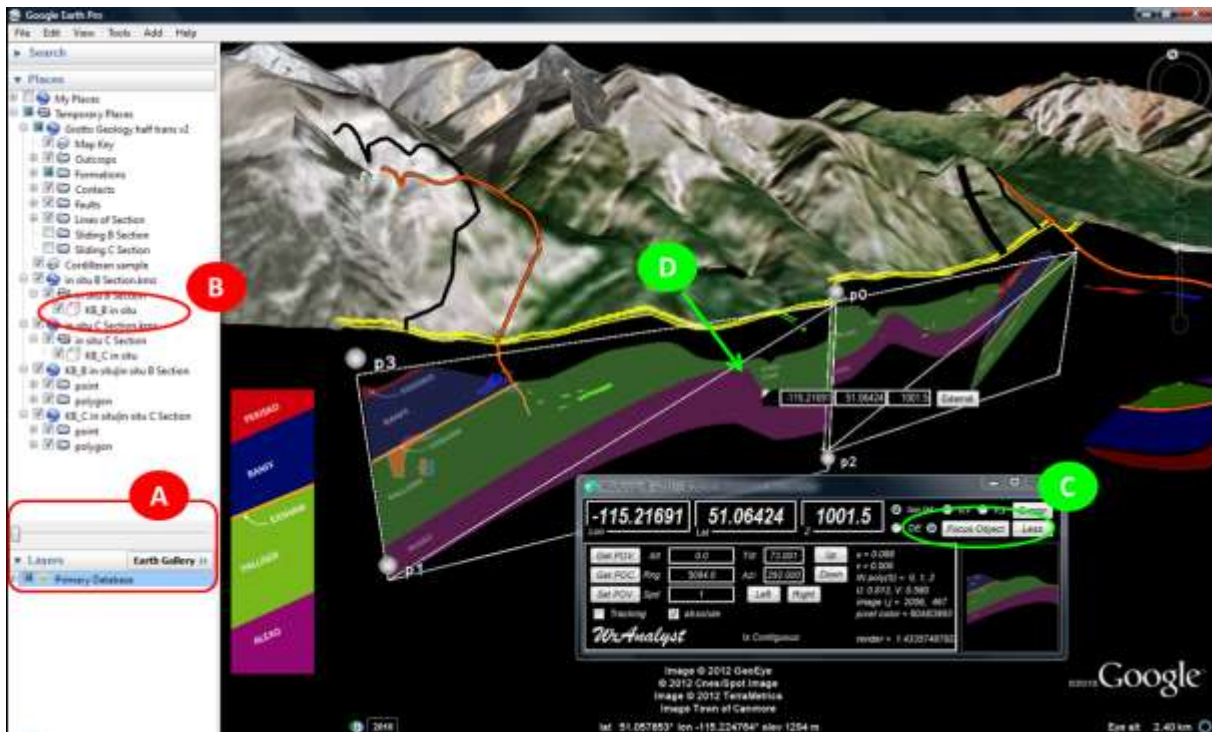
Figure 10 – WxAzygy® Tools operating in 3D on the selected COLLADA cross section. The WxAzygy interface provides the ability to “point and click” on a COLLADA surface without leaving Google Earth. This add on uses the GE COM API to interpret a user click event on the GE surface as an intersection with a COLLADA model along the user’s line of sight. Note that the coordinates of the selected point provide the real world location {long,lat} and height {metres} above the geoid, which in this example is below ground level. The ability to remove the Primary Database (“A”) is currently supported only in Google Earth 5.x and 6.0. In version 6.2, the Radar item in the Weather folder must be made transparent. User highlights the COLLADA surface (“B”), then selects that surface as the Focus Layer (“C”) and uses the geoCursor (“D”) to click on that surface.
